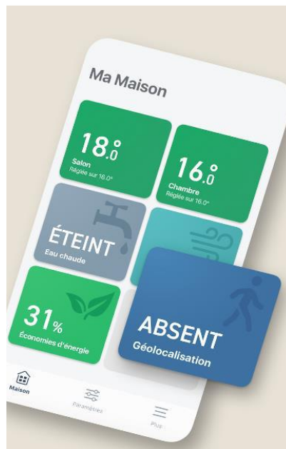
Figure 25. Tado (France) - Geolocation: the system automatically adjusts the heating or cooling settings based on your location
