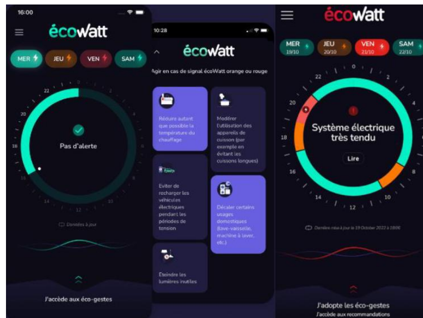
Figure 14. EcóWatt (France) – Customer tips based on electrical system state. The user can see the prevision of grid state during the following days, and its evolution during the day.
