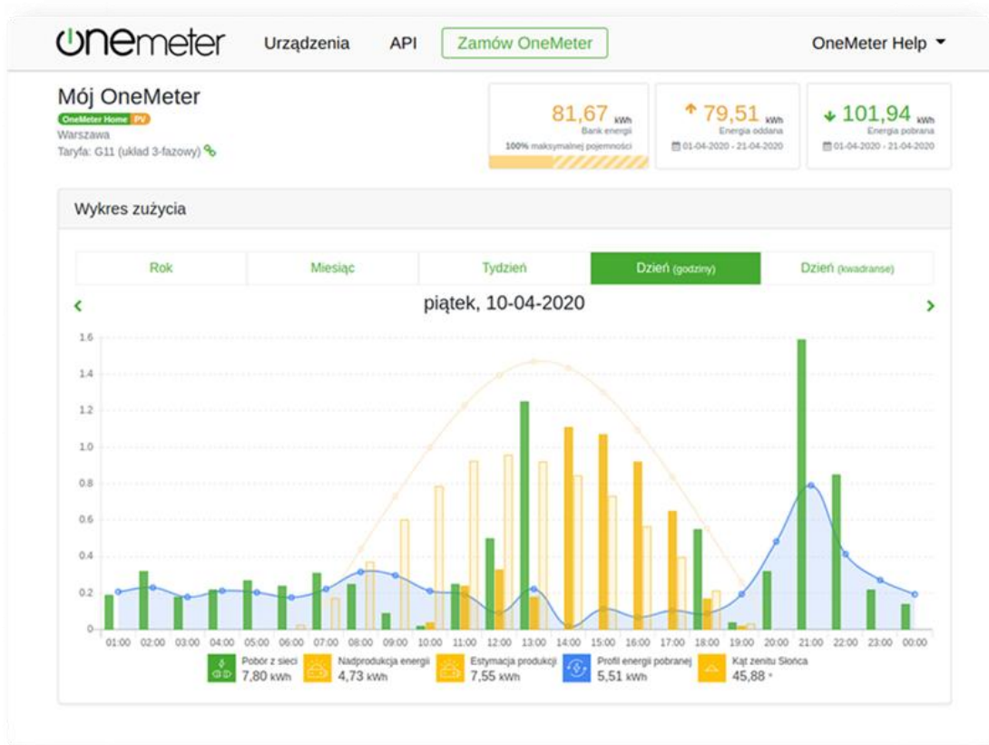
Figure 5. OneMeter (Poland) – Historical user consumption and PV generation along one day (estimated vs real).
